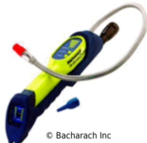
Figure 19. Refrigerant gas detectors for hydrocarbon (HC) refrigerants
