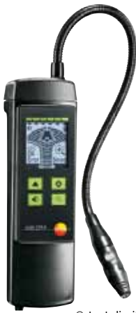
Figure 21. Refrigerant gas detector for ammonia (R-717)
